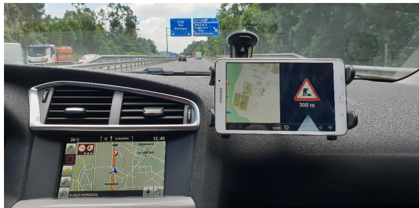
Figure 14: Different HMIs (serial-PSA- and nomadic-CTAG-) displaying same warning during a test trip
