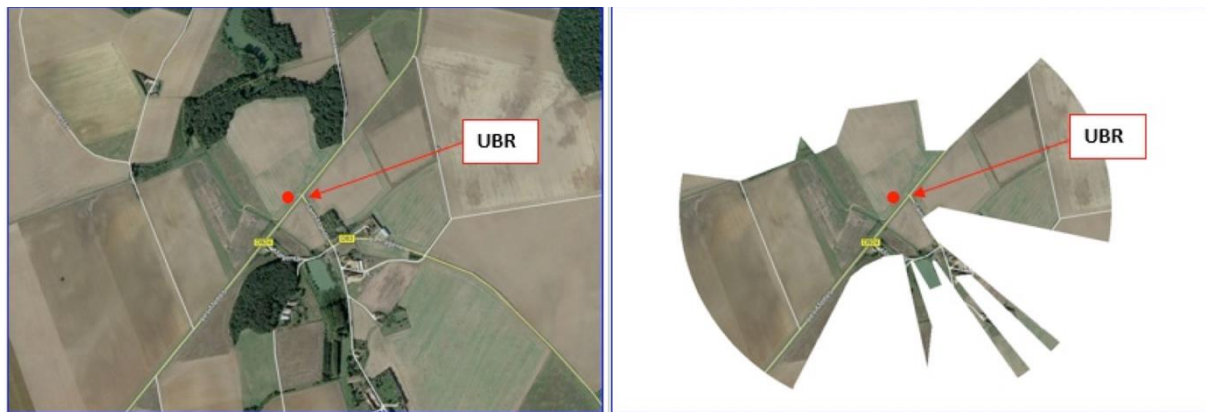
Figure 82: Example of R-ITS-S location and actual coverage area (omnidirectional antenna)
