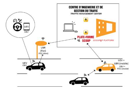
SCOOP involves both fixed Road Side Units (RSUs) and On Board Units installed in the road operator's vehicles (OBU-ro), which can act as mobile RSUs. The SCOOP central ITS station, named SCOOP Platform, links these together. It can be deployed at any Traffic Management Center (TMC) of any road operator. It is used by the 5 pilot sites involved in SCOOP, in various environments.
